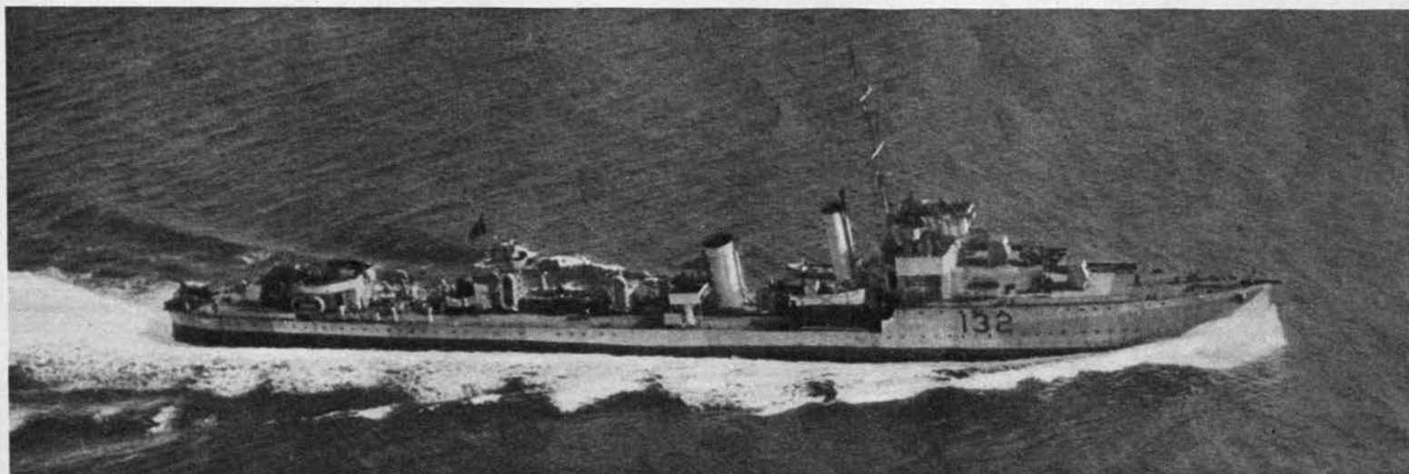
ADMIRALTY "V" CLASS Versatile has many characteristics of British ship construction: square-cut bridge, angular gun mounts, sharp-
